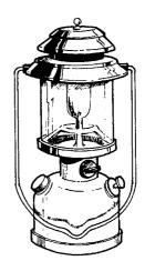
Pressure lamps - The second type of lamp, called 'pressure lamps', uses a liquid fuel which is vaporised and then burned in the same way as a gas lantern. The liquid fuel can be petrol or paraffin.
