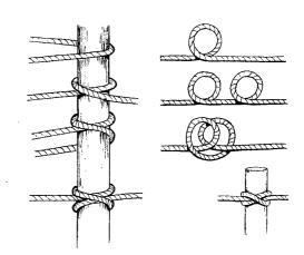
Thus the two ends of the rope should be laid next to each other under the diagonal but running in opposite directions. The clove hitch looks like a 'N'.
